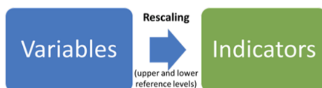
Figure 2. Example of deriving condition indicators by rescaling the values obtained for variables, based on upper and lower reference levels
